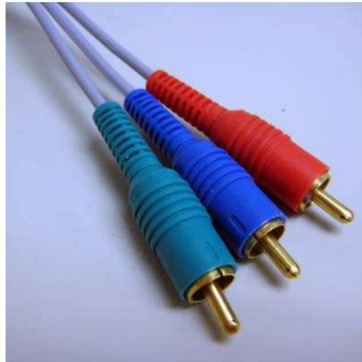
Fig. 4.1 Typical RGB Component Video Connection
